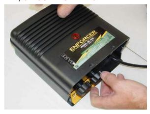
Hold down energizer with one hand then slide out inner module by pulling on knob near center (do not pull on power cord).
