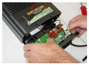
4. Most repairs need to be made by replacing the circuit board. Firmly lift the front of the circuit board up and away from the tabs holding it in.
