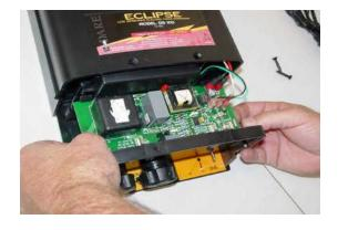
5. Slide inner guts back into place. Replace both screws. Do not over tighten. Turn on energizer, test with a volt meter, you should get a reading above 5,000 volts.
