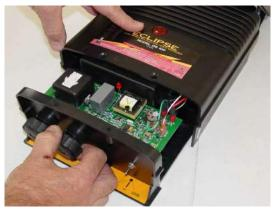
Hold down energizer with one hand then slide out inner module by pulling on knob near center.
